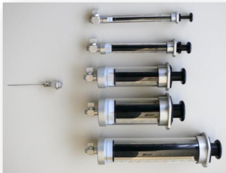
Gas-tight syringes with on/off valve
